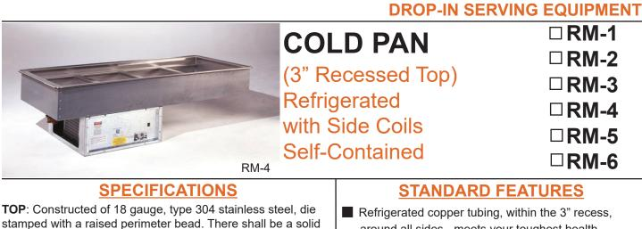
stamped with a raised perimeter bead. There shall be a solid vinyl gasket under the beaded edge to form a seal to the counter top, thus preventing seepage or marring of the counter top. Embossed mounting lugs are provided along the inner surface, 3" down from the top, to hold the pan rails and a full set of removable separator channels in place.
