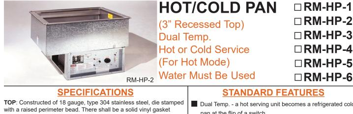
under the beaded edge to form a seal to the counter top, thus preventing seepage or marring of the counter top. Embossed mounting lugs are provided along the inner surface, 3" down from the top, to hold the pan rails and a full set of removable separator channels in place.
